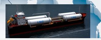
EPM2: Barge retrofit for LNG bunkering within the port
